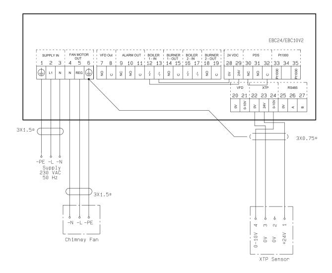
The example shows how a voltage signal (24 V DC) is connected to EBC10v2 for the chimney fan to run continuously
