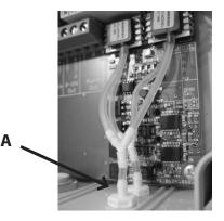
If the pressure transducer is positioned in a place where insects have access to the free end, fitting a sinter filter is recommended.
