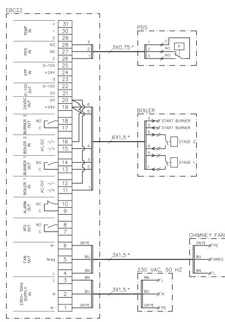
This example shows which inputs/outputs on the EBC22 need to be connected to a 2-stage boiler: The boiler outputs for stages 1 & 2 are two potential free contact sets.
