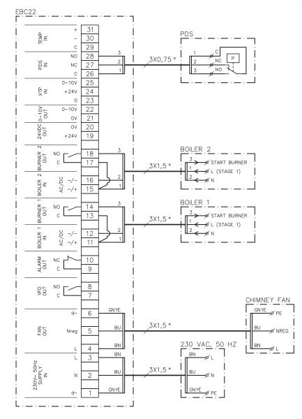
This example shows which inputs/outputs on the EBC22 need to be connected to  $2 \times 1$ -stage boilers. The boiler output for stage 1 is a voltage signal.
